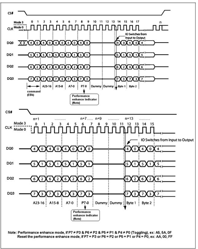
Quad Input/Output Fast Read Enhance Performance Mode Sequence in QPI Mode
