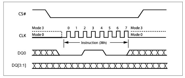
Enable Quad Peripheral Interface mode Sequence Diagram
