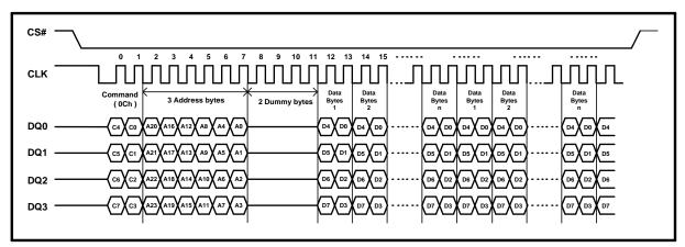
Read Burst Instruction Sequence Diagram in QPI mode
