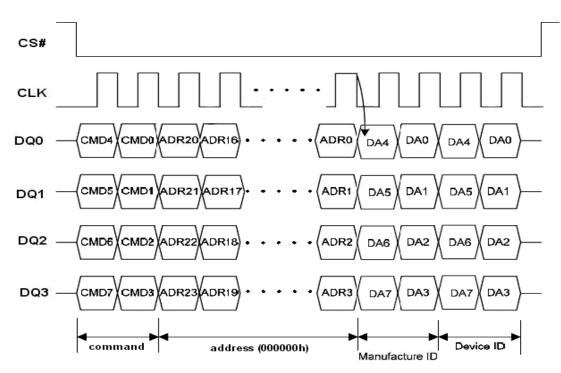
Read Manufacturer / Device ID Diagram in QPI Mode
