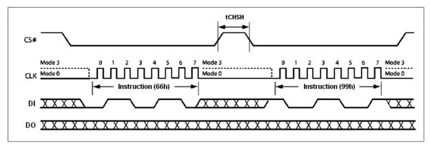
**Reset-Enable and Reset Sequence Diagram**
