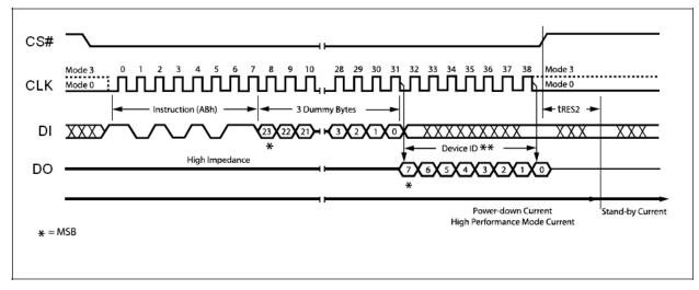
Release Power-down / Device ID Instruction Sequence Diagram
