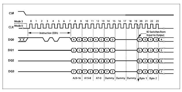
The Quad Enable bit (QE) of Status Register (S9) must be set to enable for the Quad I/O Fast read command.
