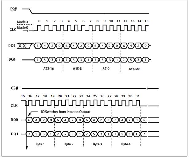
Dual Input / Output Fast Read Instruction Sequence Diagram with "Enhance Read Mode" (M5-4 = (1,0))
