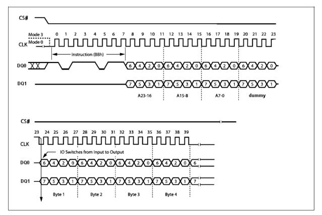
Dual Input / Output Fast Read Instruction Sequence Diagram (M5-4  $\neq$  (1,0))
