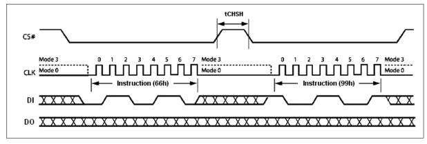
**Reset-Enable and Reset Sequence Diagram**
