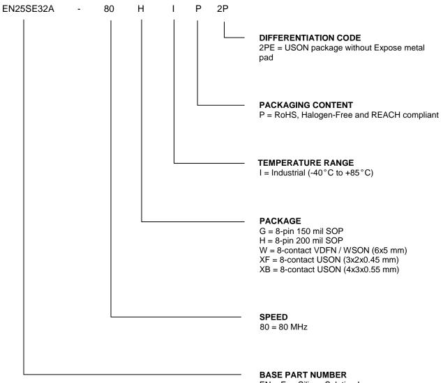
EN = Eon Silicon Solution Inc. 25SE = 1.65-1.95V Serial Flash with 4KB Uniform-Sector 32 = 32 Megabit (4096K x 8) A = version identifier
