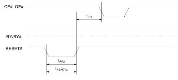
Reset Timing NOT during Embedded Algorithms
