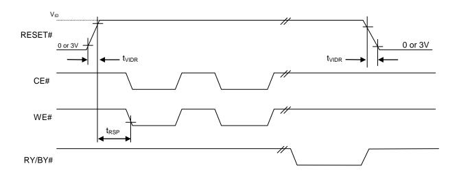
Figure 11. Sector Protect/Unprotect Timing Diagram
