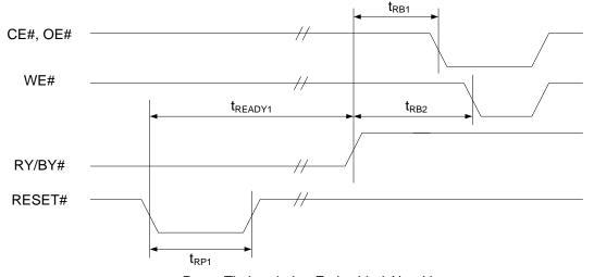
Reset Timing during Embedded Algorithms
