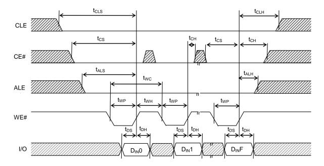
Note: DINF means the Final Data Input.
