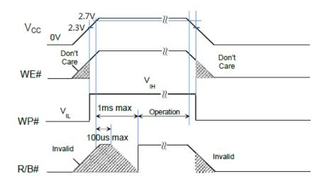
**AC Waveforms for Power on Transition**
