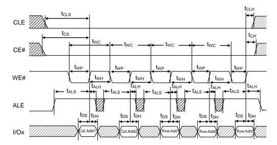
**Address Input Cycle Timing**
