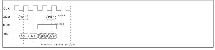
\*Note: 1. To prevent bus contention, DQM should be issued which makes at least one gap between data in and data out.
