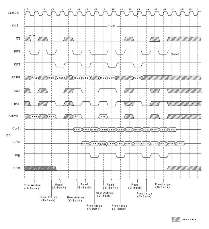
Note: 1.  $\overline{CS}$  can be don't cared when  $\overline{RAS}$ ,  $\overline{CAS}$  and  $\overline{WE}$  are high at the clock high going edge. 2. To interrupt a burst read by row precharge, both the read and the precharge banks must be the same.
