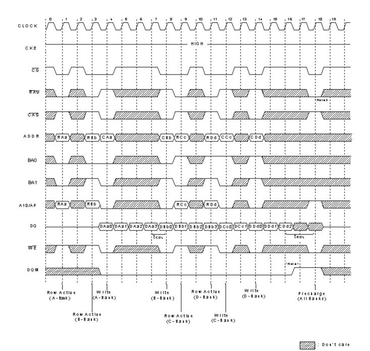
1. To interrupt burst write by Row precharge, DQM should be asserted to mask invalid input data.
