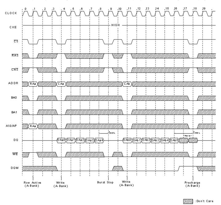
Write interrupted by Precharge Command & Write Burst Stop Cycle @ Burst Length = Full page
