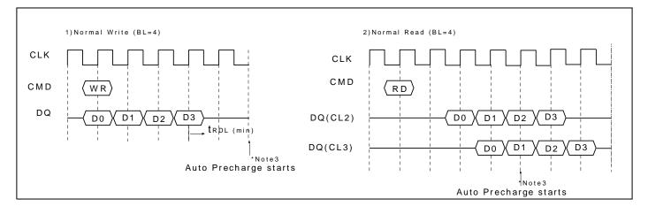
\*Note: 1. t<sub>RDL</sub>: Last data in to row precharge delay.
