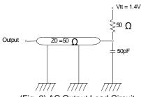
(Fig. 2) AC Output Load Circuit
