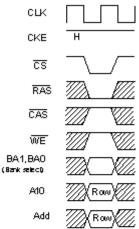
Fig. 2 Row address strobe and bank active command
