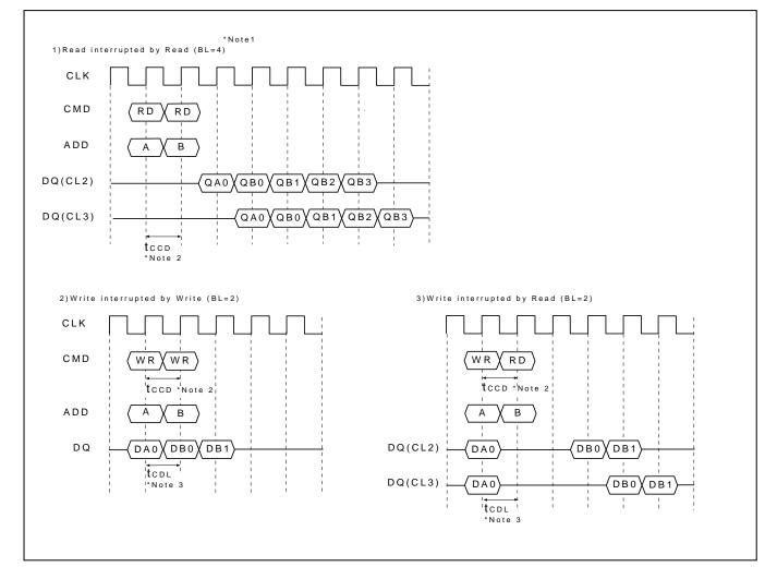
\*Note: 1. By "interrupt" is meant to stop burst read/write by external before the end of burst. By " $\overline{CAS}$  interrupt", to stop burst read/write by  $\overline{CAS}$  access ; read and write.
