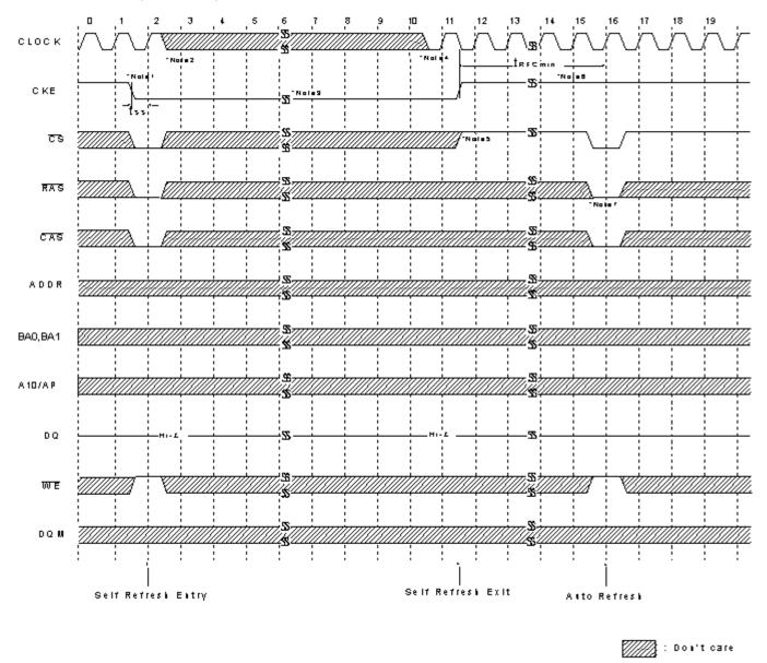
\*Note: Self refresh mode is not supported for VA grade with  $T_A{>}85~^\circ \!\!\!\mathrm{C}.$
